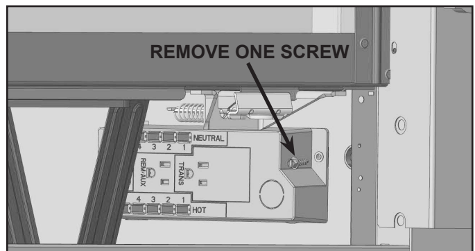
Figure 8.3 Junction Box Detail - JADE32IN-B
